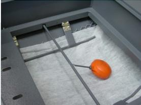
As the filter cake builds up it impedes the flow of medium, thus causing the fluid level in the filter trough to rise until a float switch is actuated. As a result, the float switch activates the feed belt and a
